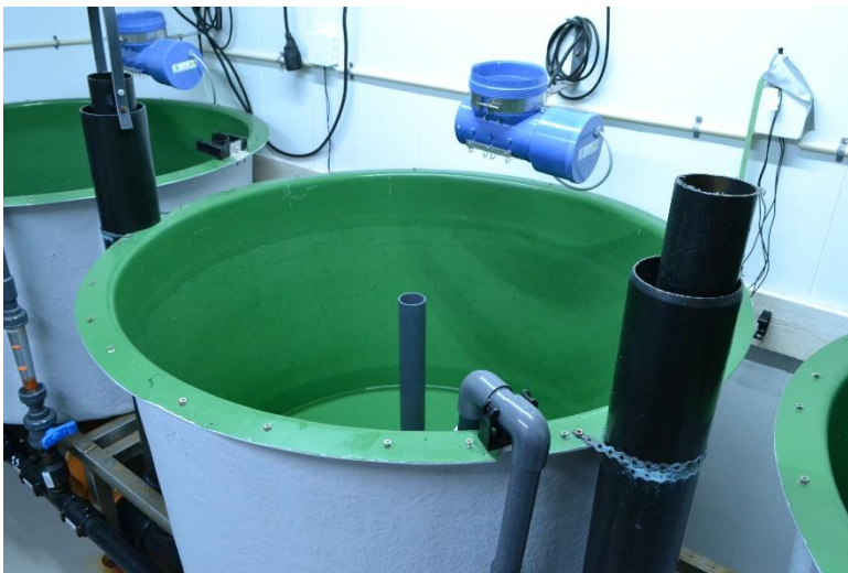
Figure 1: Standard fiberglass on-growth tank with Arvotec feeders and below-surface water inlet. A deep tank as shown in the figure is not required. Any smooth flat-bottomed tank is technically suitable for the on-growth phase.
